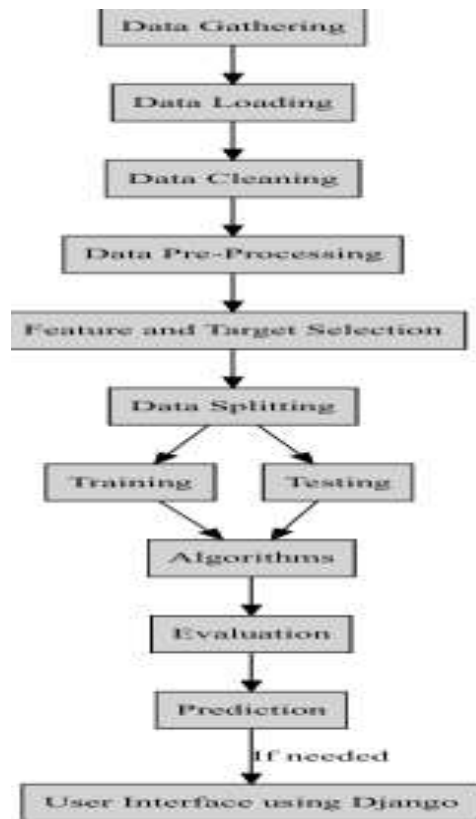
Fig: 3.1 Flow diagram for Machine learning pipeline
